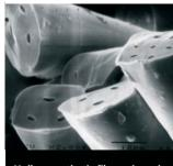
Hollow synthetic fibres viewed under a scanning electron microscope (SEM). © IFTH
