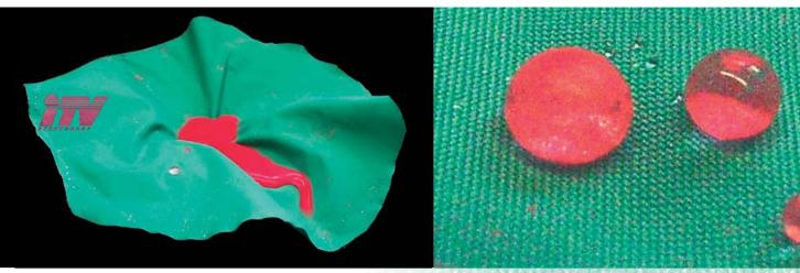
The self-cleaning and hydrophobic properties of textiles manufactured using the nanotechnological process known as the Lotus effect®. @V.v.Arnim-ITV Denkendorf
