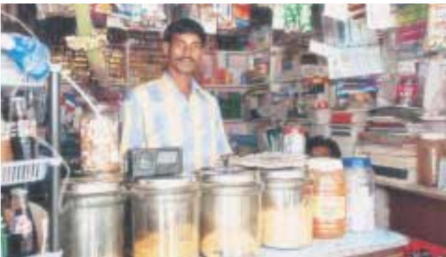
The modified radio set in use at a local shop in Budikote's small market area on the main street; The co-axial cable (coming from the upper left of the photograph) carrying the Namma Dhwani FM signal connects to the radio through a specially modified jack. For those that have them, audience members can also listen to the radio programmes through their television sets. One of the many beauties of radio, listeners are able to listen while they carry on with their everyday activities. Photo credit: Santosh.H.S. / Namma Dhwani / VOICES
