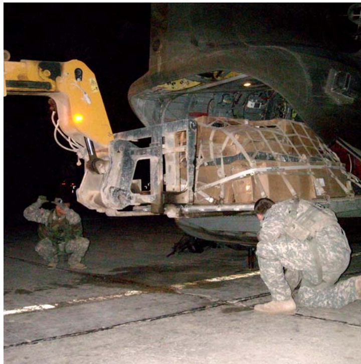
Figure 3. Pallets are used for cargo too large or heavy for a triwall. Pallets require a forklift for loading and eliminate adjacent passenger seating on helicopters.
