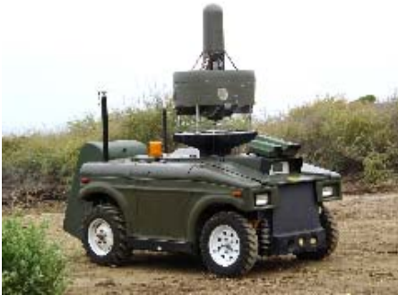
Fig. 5. Example of ducted fan UAV [11].
