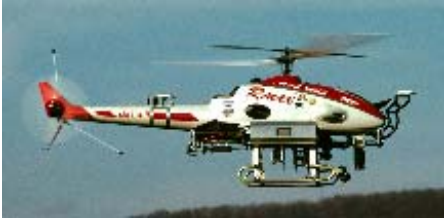
Fig. 4. Aerial mapping platform: CMU Autonomous Helicopter.
