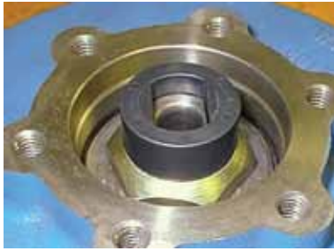
Figure 1 Pulley hub with coupler in place on shaft (Figure 1)
