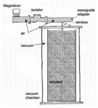
Our current experimental setup has the vacuum system contained in a -77C scientific freezer that can simulate Martian conditions. Microwaves are delivered down a borehole to depths where water ice could be present. Heating at progressively deeper levels within the borehole would permit the determination of water concentrations with depth. Calculation of volatile mass flow rates is being developed to use with existing numerical models.
