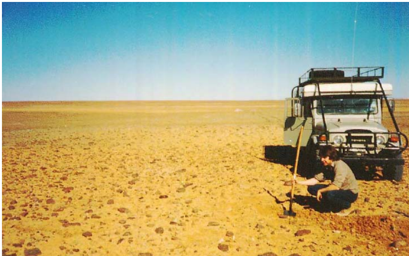
Figure 3. Surface cover of gibber lag and silty clay (Benitos Clay) over epsomite deposit. From [20].
