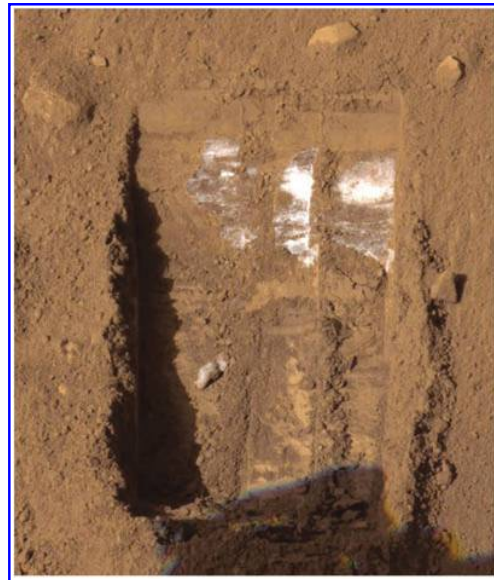
FIG. 39. Near-surface ground ice uncovered at the PHX landing site. The image shows the 22 cm wide, 35 cm long, and ~7–8 cm deep “Dodo-Goldilocks” trench after two digs by the PHX robotic arm. Image credit: NASA/JPL-Caltech/University of Arizona/Texas A&M University.
