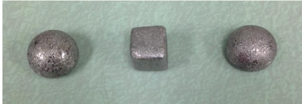
(a) 1.5% wt B (b) 1.5% wt BN (c) 1.5% wt BC Figure 9: The Distorted Samples After Sintering at 1250°C
