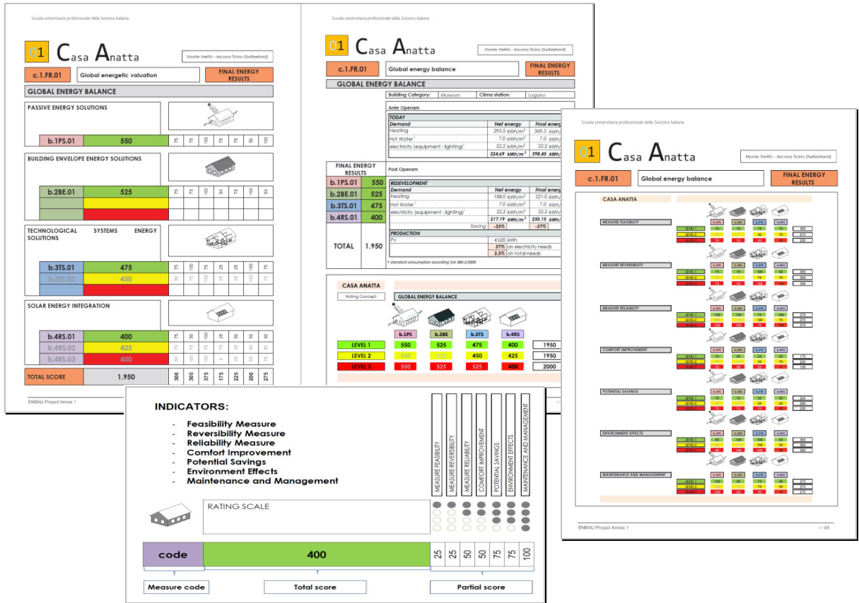
Fig. 6. Global energy assessment chart (third step c). This chart summarizes all the proposed solutions and allows a tangible and clear overview of the benefits brought to the building by the proposed solutions.
