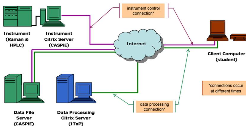
Figure 1. Schematic of instrumentation network.
