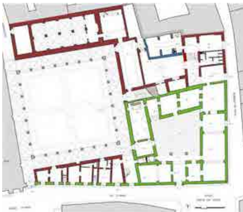
Image 1: Ground floor of the Saint Anne Convent in Palermo. In green: XV-XVI century stone walls. The calcarenites came from intra moenia quarries. In red: XVII-XVIII century structures, where calcarenites from extra moenia urban quarries was used. In blue: mid XIX century masonry, made of calcarenites from coastal areas (Aspra). (On the basis of the project plan: De Angelis Ricciotti, D., Li Castri, M., & Martelli, T., "Progetto di completamento")
