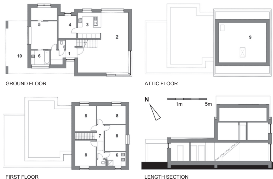
Fig. 3 Selected case Wienerberger/Recticel project; 1. entrance hall/toilet/checkroom 2. living room 3. kitchen 4. pantry 5. main double bedroom/office space 6. bathroom 7. landing 8. single bedroom 9. attic 10. carport (design: arch. Cauchie).
