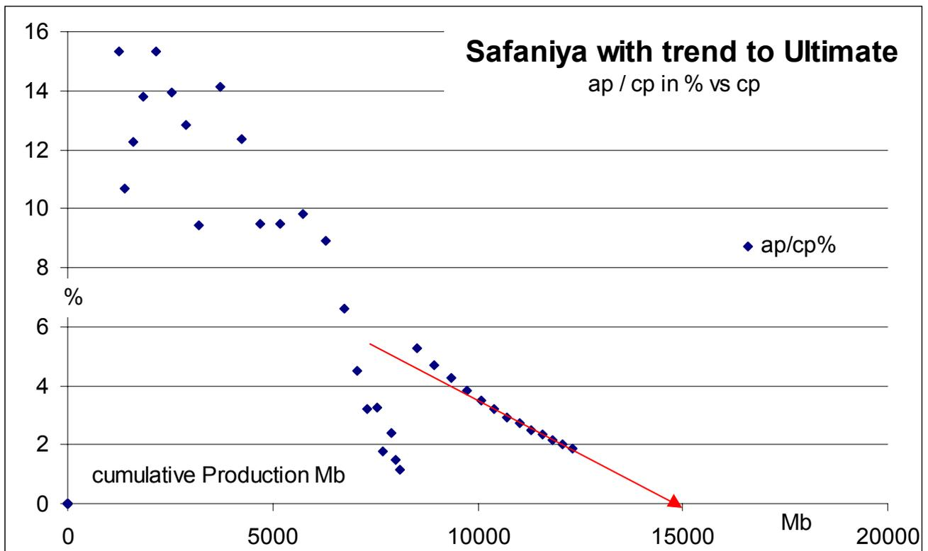
**Figure 15:** Safaniya seems to have a EUR about 15Gb; cp end 2003 is about 12.5Gb. It is not excluded, that the field was produced at higher rates especially after 1998, but we have no data, confirming this. The hints are: relatively small "26% of reserves produced" (CSIS 2004 giving 48Gb OOIP, recovery factor 31.2%), as well as the difference to the off-shore-Industry-statistic (flat) and the great range of claimed production-capacity: 500-600kb/d (Simmons) vs. 1500kb/d (Cordesman & Obaid).
