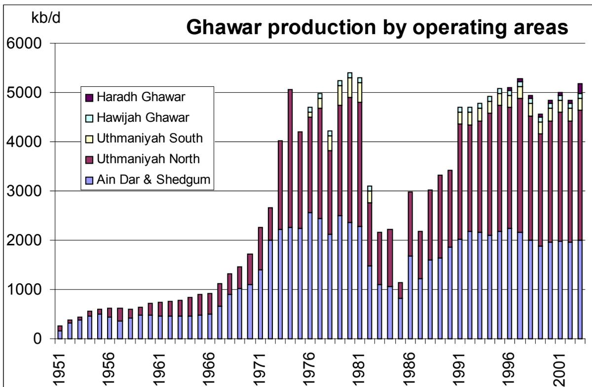
**Figure 2:** this graph shows the importance of the sweet spots 'Ain Dar and Shedgum (source Baqi & Saleri) and Uthmaniyah North of the Ghawar field (modelled by jud). The publication of Saudi Aramco officials allowed to design solid graphs pointing to the Ultimate the different parts of the Ghawar field will probably be able to produce:
