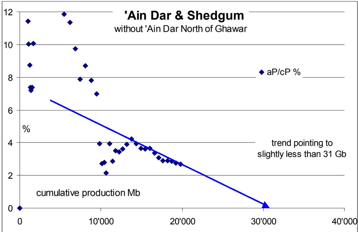
**Figure 4b:** Second: 'Ain Dar & Shedgum Area LESS 'Ain Dar North Baqi & Saleri claim in 2004 that proven reserves are 40.8Gb (60% of OOIP). Based on past production-analysis this is EUR; 60% rf is very high and the oil is still in the ground! It is a great challenge to produce it already today, and it will be a even greater in future.
