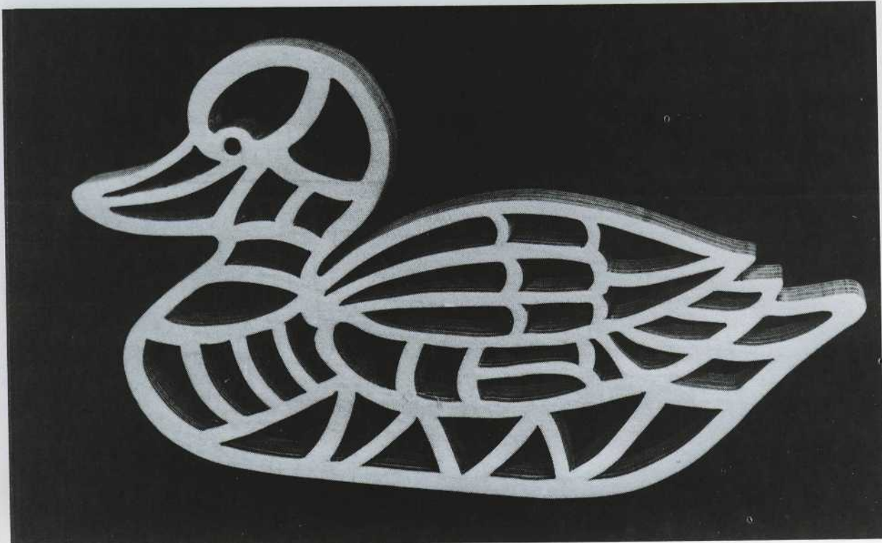
Fretted duck sawn from 1/2-inch thick Baltic-birch plywood.
