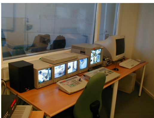
Figure 4. Control room: equipment for operating the motorized video cameras in the subject room.
