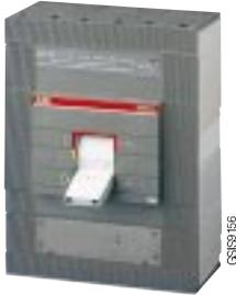
**S6D 400**  $I_u (40\text{ °C}) = 400\text{ A}$   $I_{cw} (1s) = 15\text{ kA}$   $I_{cm} (415\text{ V}) = 30\text{ kA}$
