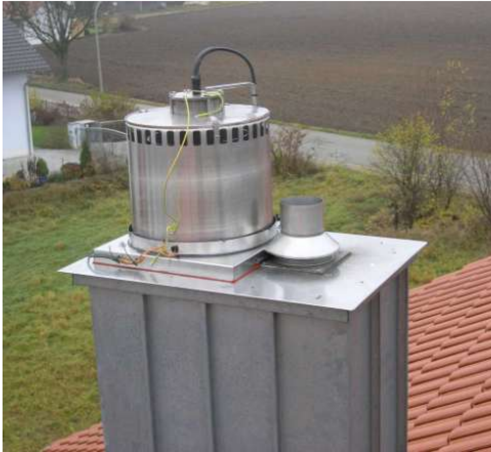
APP R esidential ESP, example here: with chimney stove (6 kW)
