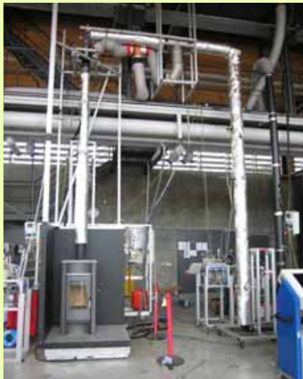
Dilution tunnel at TFZ
