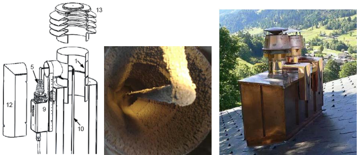
Figure 25: Scheme of the OekoTube technology (left), picture of electrode (middle) and picture of mounted ESP (right)
