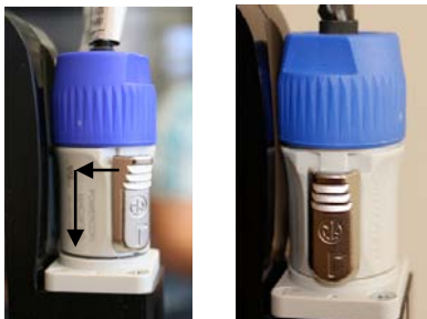
Fig. 88: Inserting the connector plug
