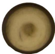
Fig. 10: Filter cartridge visibly loaded
