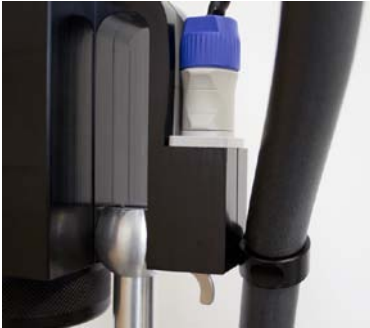
Fig. 6: Fastening the intake hose holder
