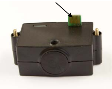
Fig. 93: Sensor module with pinboard
