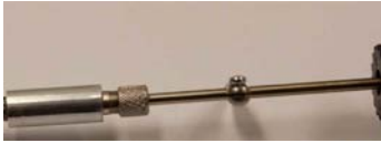
Fig. 71: Particulate-matter sampling probe connected to the heating hose
