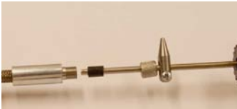
Fig. 74: Rubber seal at the end of the sampling probe
