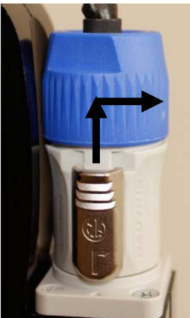
Fig. 82: Releasing and twisting the connector plug
