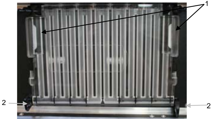
Fig. 62: Close-up view of the flue gas condenser
