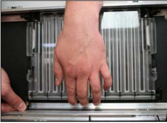
Fig. 65: Refitting the condenser
