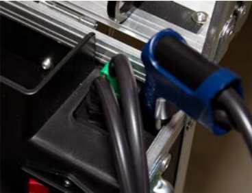
Fig. 12: Connecting the probe and cable-hose assembly
