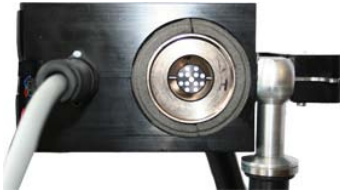
Fig. 78: Filter holder and filter cartridge
