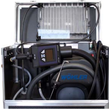
Fig. 15: Intake hose coiled around the reel
