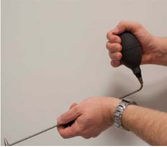
Fig. 73: Cleaning the sampling probe
