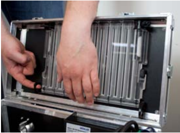
Fig. 63: Removing the flue gas condenser
