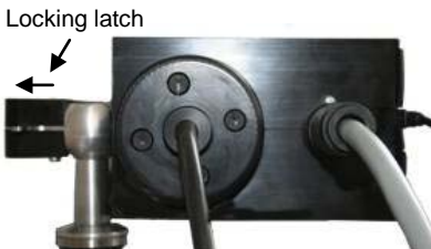
Fig. 5: Undo the locking latch on the digital mass scale unit
