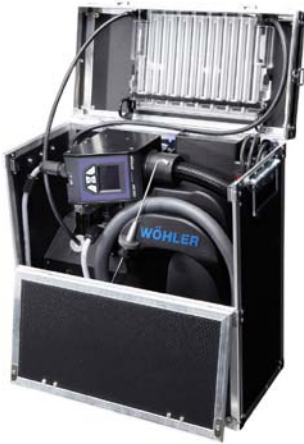
Fig. 7: Analyser components stowed in case
