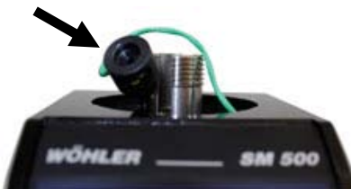
Fig. 85: Hose temperature sensor
