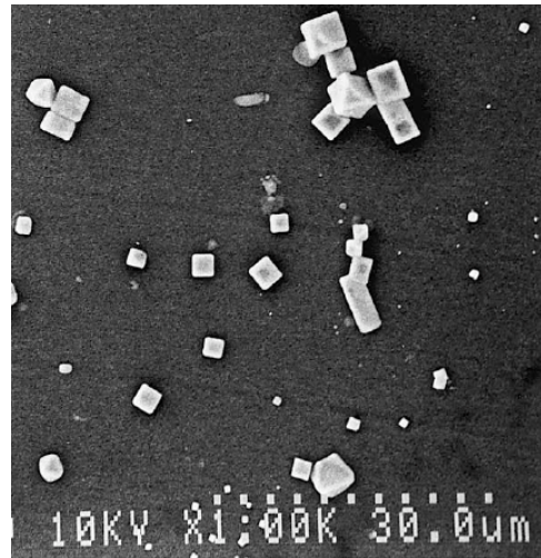
Figure 1.5 SEM-pictures of particles in the flue gas of an automatic wood combustion system. Left is the combustion of wood resulting in submicron particles. Right is the combustion of herbage grass resulting in larger particles at higher mass concentrations [Kaufmann et al. 2000].
