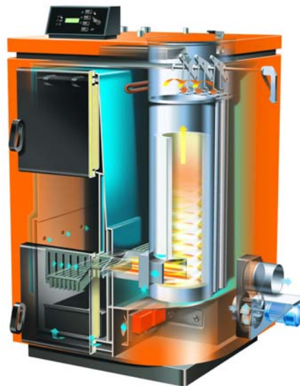
Figure 2.13 Downdraft boilers with inverse combustion of log wood and with enforced air flow and air supply with primary and secondary air. Graphs: [Nussbaumer 2003], bottom right: Schmid AG Eschlikon.
