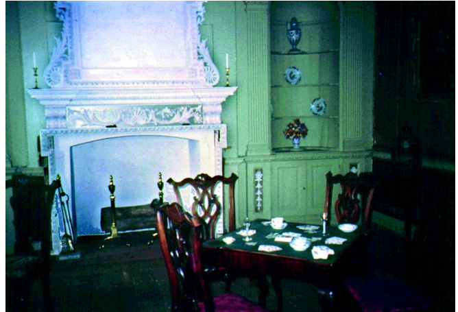
Figure 7: Ducted central HVAC systems have been used in a compatible way at Gunston Hall in Virginia, the 18 th century home of George Mason. As seen in this view, there are no dropped bulkheads, soffits, or ceiling registers to disfigure the elegance of this historic room. The chimney serves as a supply. This house museum has a stable furnishing collection, and the HVAC is not fitted with humidification. In winter, the relative humidity occasionally drops below 25%, but monitoring does not reveal that the collection is being damaged. The house stays heated in winter because the docents are in the house during the day. Special fragile collections are exhibited in the climate-controlled visitors center.
