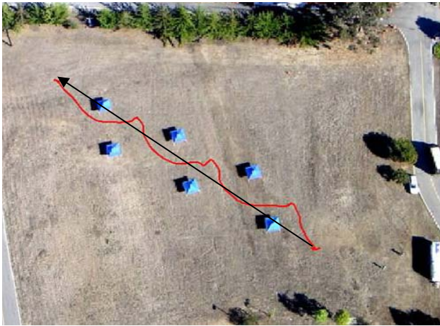
Figure 6. Aerial view of urban experiment (black: given straight path, red: actual flight path of UAV during experiment)
