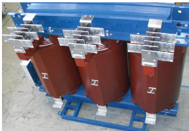
Fig. 5.9-12: 4771 kVA GEAFOLE converter transformer with 5 secondary windings 10/0.33 – 2.4 kV
