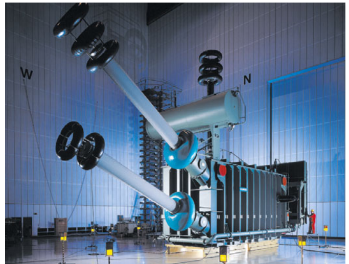
Fig. 5.8-2: Converter transformer for HVDC bipolar transmission system \pm 500 kVDC; 2,500 MW: single phase; 420 kVAC; 515 kVDC; 397 MVA; wye system (left side of figure) and delta system (right side of figure)
