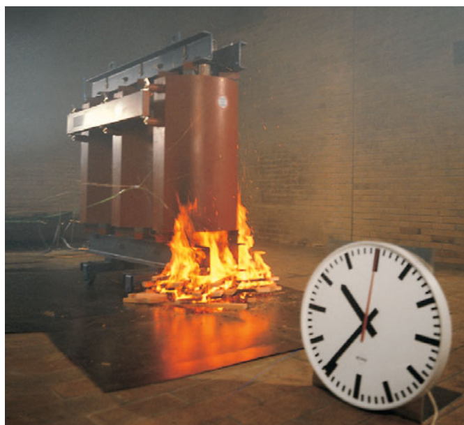
Fig. 5.9-6: Flammability test of cast-resin transformer
