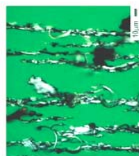
Cutting Wear on a Ferrogram
