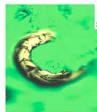
Figure 7. These Ferroglyphic Images are Typical of the Shape of Wear Particles Produced by Three-body Abrasive Wear.
