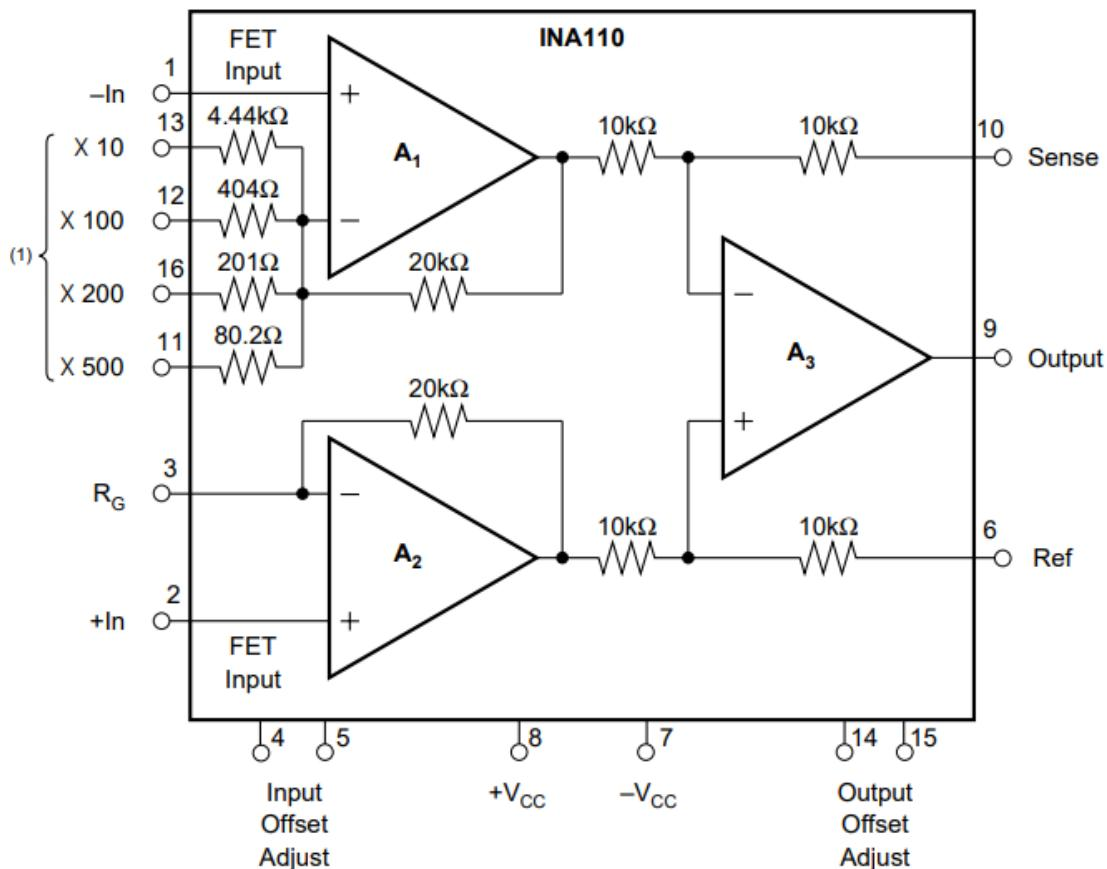
NOTE: (1) Connect to R<sub>G</sub> for desired gain.
